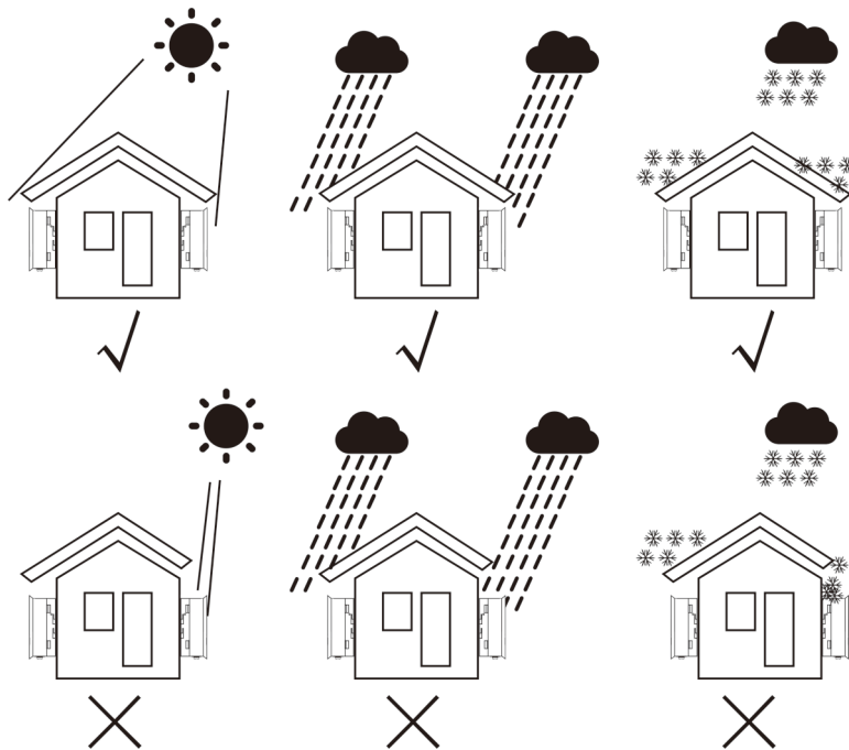
Figure 4.1 Recommended Installation locations
