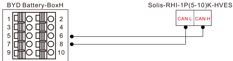
Figure 4.12 BYD Battery Communication
