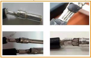
**Solution:** Use an MC4 wrench to remove the DC connector and crimp the DC terminal again.
