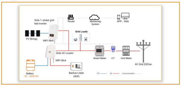
This solution is a better choice for users who have already installed photovoltaic systems. In addition to AC-coupled inverters and energy storage batteries, no additional equipment and costs are required. The installation circuit only needs to be simply modified in the original power distribution test. The storage capacity of the system depends on the capacity of the battery pack, which can provide power for key loads of about 3kW without interruption when off-grid.
