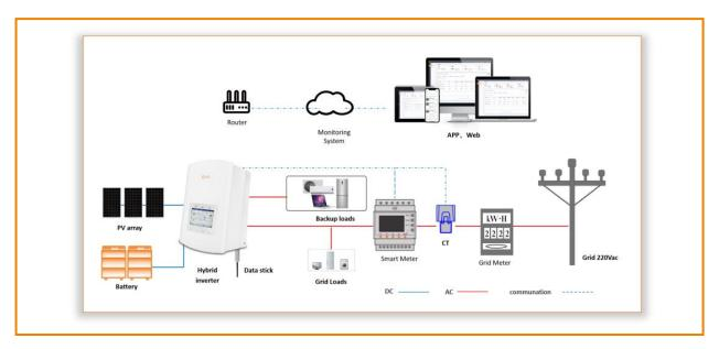
By constructing a hybrid inverter + energy storage battery power supply system, the entire photovoltaic system can be guaranteed to operate at any time, stably and effectively supplying important household loads. If you need to use three-phase power or the household electricity load is large, you can also use a three-phase energy storage system.
