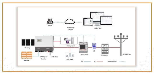
The above solution is suitable for newly-added photovoltaic systems. If a photovoltaic system is already installed, the inverter can also be replaced with a photovoltaic hybrid inverter and other power supply side circuit modifications under the condition that the original main circuit remains unchanged. This modification method It will undoubtedly increase certain difficulties.
