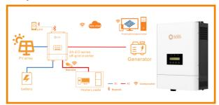
This off-grid solar + energy storage system is mainly comprised of solar panels, batteries, off-grid energy storage inverter(s), loads and can also be connected diesel generators. This system will mainly be used in areas where the grid is unreliable or there is no power grid at all. The system can directly charge the battery from the solar through DC-DC conversion and can also realize bidirectional DC-AC conversion for charging and discharging of the battery.
