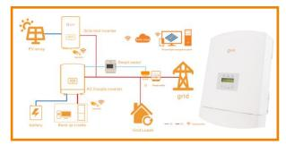
AC coupled solar + energy storage is the solution for any existing solar PV system looking to upgrade to energy storage. This system structure consists of mainly solar modules, existing grid-connected inverter(s), AC-coupled energy storage inverter(s), batteries, grid-connected loads and back-up (critical) loads. The system uses AC coupling to transform the basic grid-tied PV system through the AC side into an energy storage solution.
