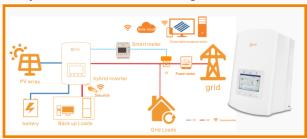
A hybrid solar + energy storage system consists mainly of solar panels, batteries, hybrid inverter(s), grid-connected loads and back up (critical) loads. The system can directly charge the battery from the solar through DC-DC conversion and can also realize the bidirectional DC-AC conversion for charging and discharging of the battery.
